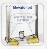
Installation effect of guide rail oiler - Flat oiler
